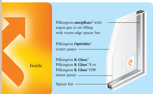
Cross section Pilkington energiKare™ unit
